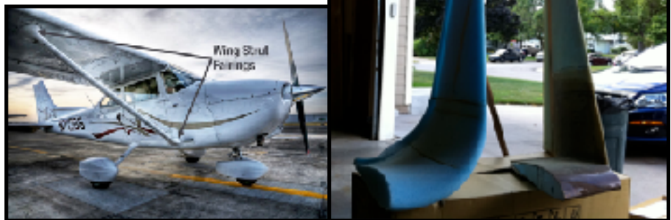
Figure 11 Interference Drag Minimization
